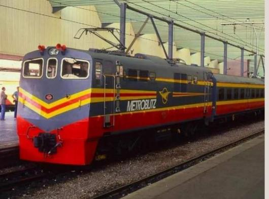
The pantographs were being considered for use on the Class 6E1 locomotives and could support speeds over 145km/h on catenary that typically only handled speeds up to 80km/h.
