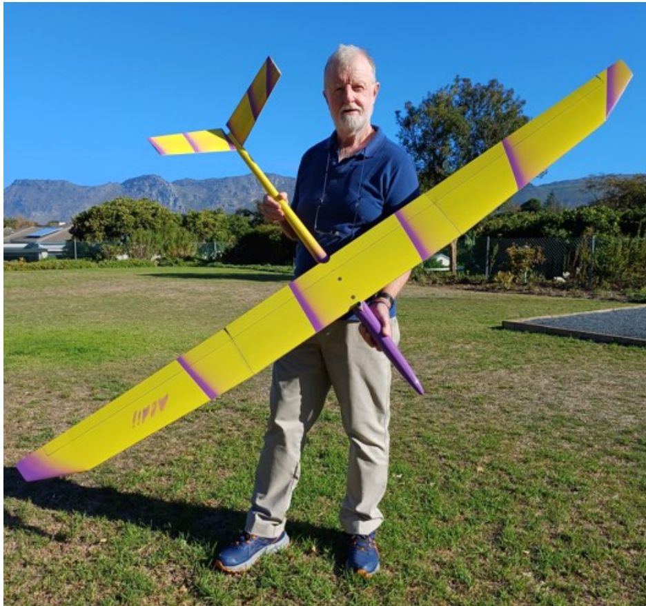
"The Aldij Slope Soarer is fibreglass and has a wingspan of 2.2m." Jim
