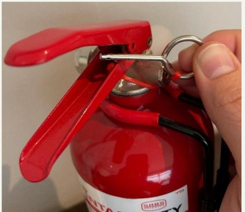
With the plastic seal removed, pull out the metal pin.
